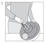
Turn the three screws firmly, but without destroying the thread. To reach the desired height, repeat this step or reverse it.
