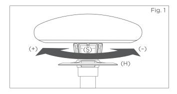
seat. With a counterclockwise rotation the tilt is reduced (-) and with a clockwise rotation increases the tilt (+), see Fig. 1. The ONGO\*Roll operates without a flexible seat.
