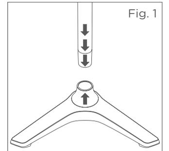
It is important that the seat is positioned in an accurate line with the foot. This is important because the gas spring will automatically be reset in one direction. Therefore, an alignment correction can only be made through releasing one of the cones. If this becomes necessary we recommend tapping the underside of the seat with a hammer while pulling on the cone holder until it is possible to loosen and re-align the seat. Under no circumstance however use force on the gas spring!
